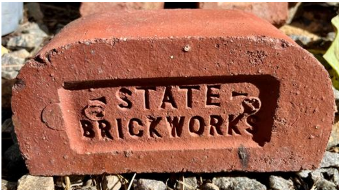
Figure 5: Double bullnose brick manufactured by the State Brickworks in the 1930s
